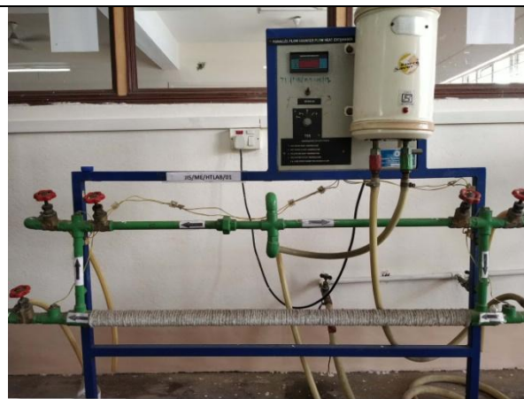
Parallel and counter-flow Heat Exchanger
